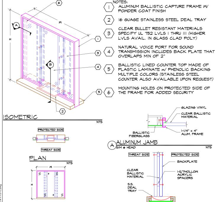
TRANSACTION WINDOW WITH VERTICAL VOICE PORT. SPECIFY LEVEL OF PROTECTION. SIZES AVAILABLE UP TO 8'W x 5'h.
