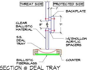
TRANSACTION WINDOW WITH HORIZONTAL VOICE PORT. SPECIFY LEVEL OF PROTECTION. SIZES AVAILABLE UP TO 8'W x 5'h.
