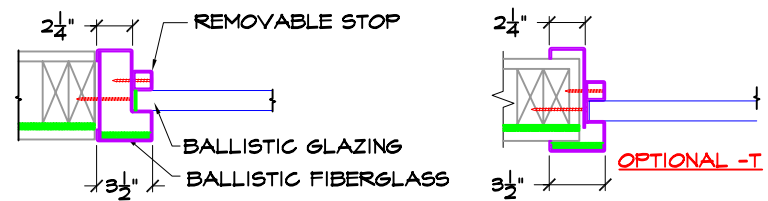
A STEEL WINDOW JAMB
